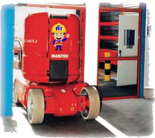
Very compact with an overall width of only 1.2m and a stowed height of less than 2m enables the 120 AETJ to access any building fitted with standard doorways.
