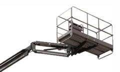
The Manitou 160 ATJ+ diesel-powered articulated platform has a load capacity that is unique on the market: 400kg. It can hold 3 operators and up to 160kg of material. It has an up and over clearance of 7m and provides a working height of up to 16.25m and a horizontal outreach of more than 10m.
